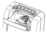
3. Blow any paper dust off the print head and from the inside of the clock using a can of compressed air. This could help prevent ribbon or card jams. Carefully insert a new cartridge, positioning the ribbon between the plastic ribbon guide and the stainless steel print shield. Push the cartridge down until it clicks into place. Turn the ribbon knob clockwise to remove any slack in the ribbon. Slide the program switch back to "Run".
