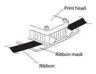
NOTICE: Install the cassette so that the ribbon is between the print head and the ribbon mask. Printing will not come out properly if the ribbon is placed behind the ribbon mask.
