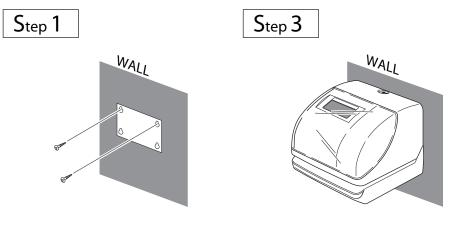
Install the supplied wall-mount screws into a wall by using the template. Be sure to keep about 6mm(1/4") of the screw head away from the wall. The recommended height from the floor to the bottom of the ES700 is 45". Replace cover and lock.
