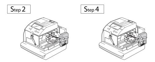
Hold the ribbon cassette by its tab and pull straight out to remove it.
