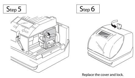
Turn the knob of the cassette in the direction of the arrow to tighten the ribbon.
