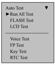
These options allow the testing of each portion of the terminal in order to pinpoint failures.
